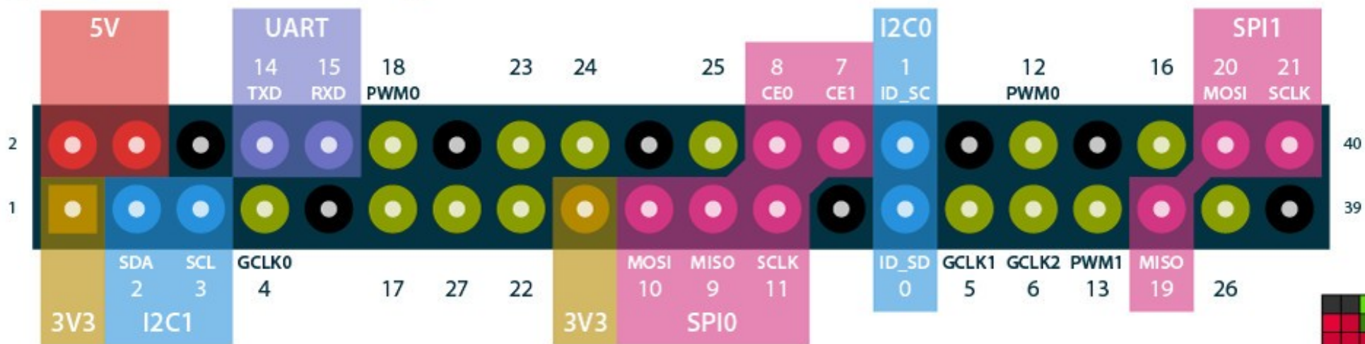
Raspberry Pi GPIO BCM numbering
